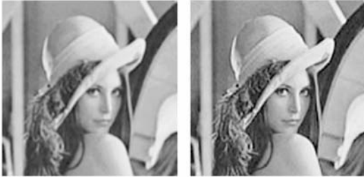
(c) 改进 Boltzmann 复原图 (PSNR=28.19 dB) (d) 本文算法复原图 (PSNR=28.64 dB) (c)Improved Boltzmann restoration image (PSNR=28.19 dB) (d)Image restored by proposed algorithm (PSNR=28.64 dB)
